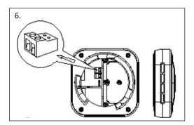
6. Plug the contacted terminal block back into the contact pin (Pic.8).
